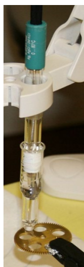
Fig. 2: The measuring system RE / junction tube.
