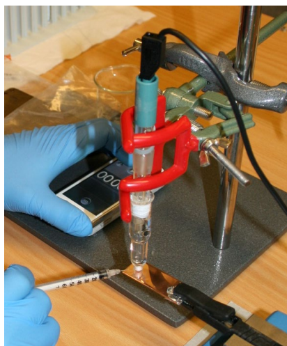
Fig. 3: Use of a syringe to insert a constant volume of solution between the RE/junction tube and the metal surface.
